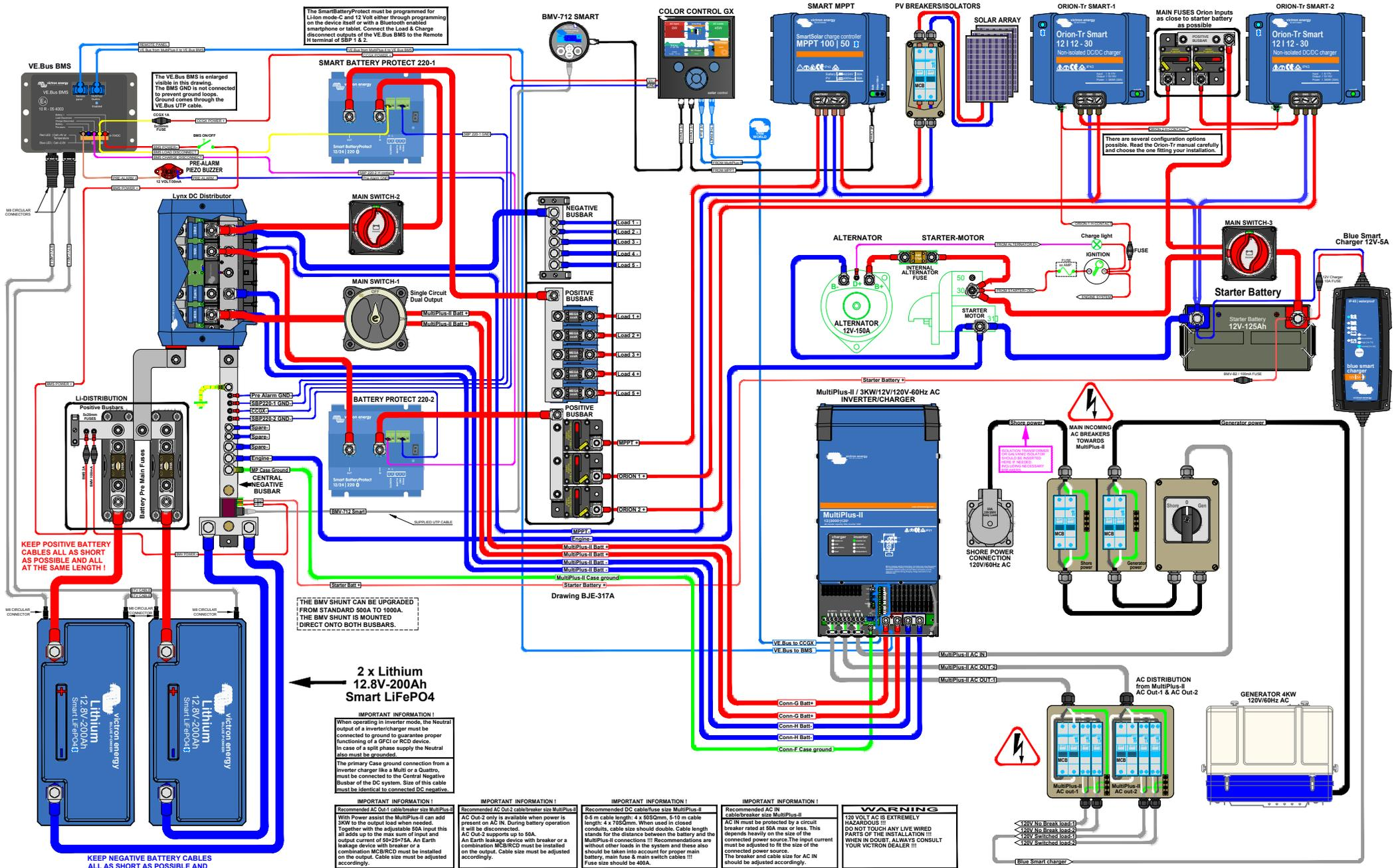
The SmartBatteryProtect must be programmed for Li-ion mode-C and 12 Volt either through programming on the device itself or with a Bluetooth enabled smartphone or tablet. Connect the Load & Charge disconnect outputs of the VE.Bus BMS to the Remote H terminal of SBP 1 & 2.
