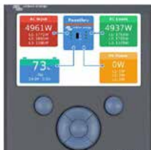
Color Control GX, showing a PV application
